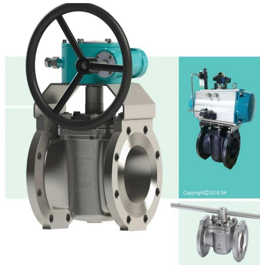
RTC non-lubricated and sleeved plug valve is designed for the most corrosive and severe chemical services. This plug valve contains a polymeric sleeve, which is inserted in the valve body. The tapered and polished plug acts like a wedge and presses the sleeve against the body. The PTFE sleeve has a low coefficient of friction and it acts as a lubricant to reduce friction between the plug and the body. This cavity-free design provides a tight shutoff with positive seal.
